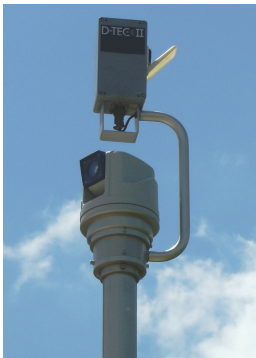
Vertical telescoping mast with camera and D-TEC II Safety System
